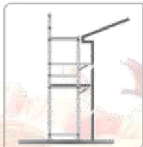
Figure 14(a): Scaffolding platform at edge of roof with hop-up bracket for other trades.
