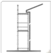
Figure 14(c): Scaffolding platform below edge of roof.
