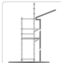
Figure 14(e): Inside standards supporting guardrailing with hop-up bracket for other trades.
