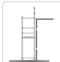
Figure 14(f): Inside standards supporting guardrailing adjacent to a flat roof structure.
