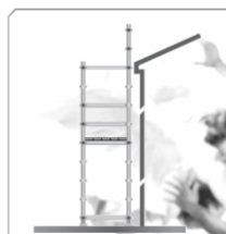
Figure 14(b): Inside standards supporting guardrails.
