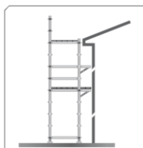
Figure 14(a): Scaffolding platform at edge of roof with hop-up bracket for other trades.
